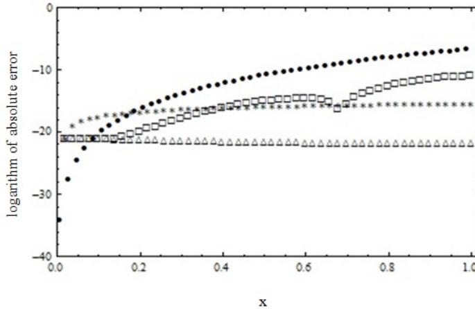
FIGURE 2. The logarithm of absolute error for three models introduced in Example 2, i.e. the usual Adams-Basforth method ( $\star$ ), the weighted model of Adams-Basforth for  $m = 5$  ( $\square$ ), the weighted model corresponding to the exact solution ( $\triangle$ ) and finally  $Q_5^{(2)}(x)$  ( $\bullet$ ) with  $h = 0.01, s = 2$  and  $m = 5$ .)
